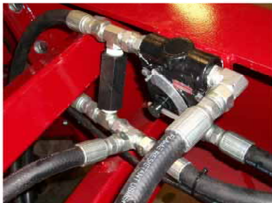
Hose routing with flow control valve
