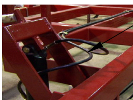
Route hoses behind tower
