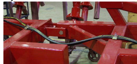
Leave a droop in hose at wing hinge.
